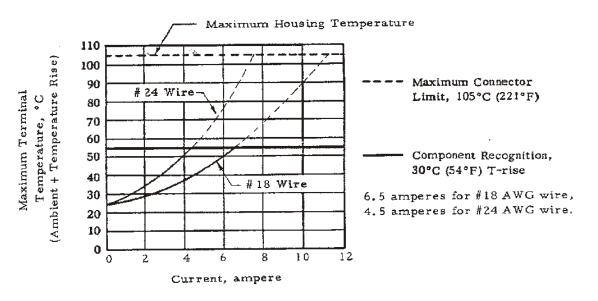
Figure 4 Terminal Temperature vs Current/Circuit, 5 Position Housing
