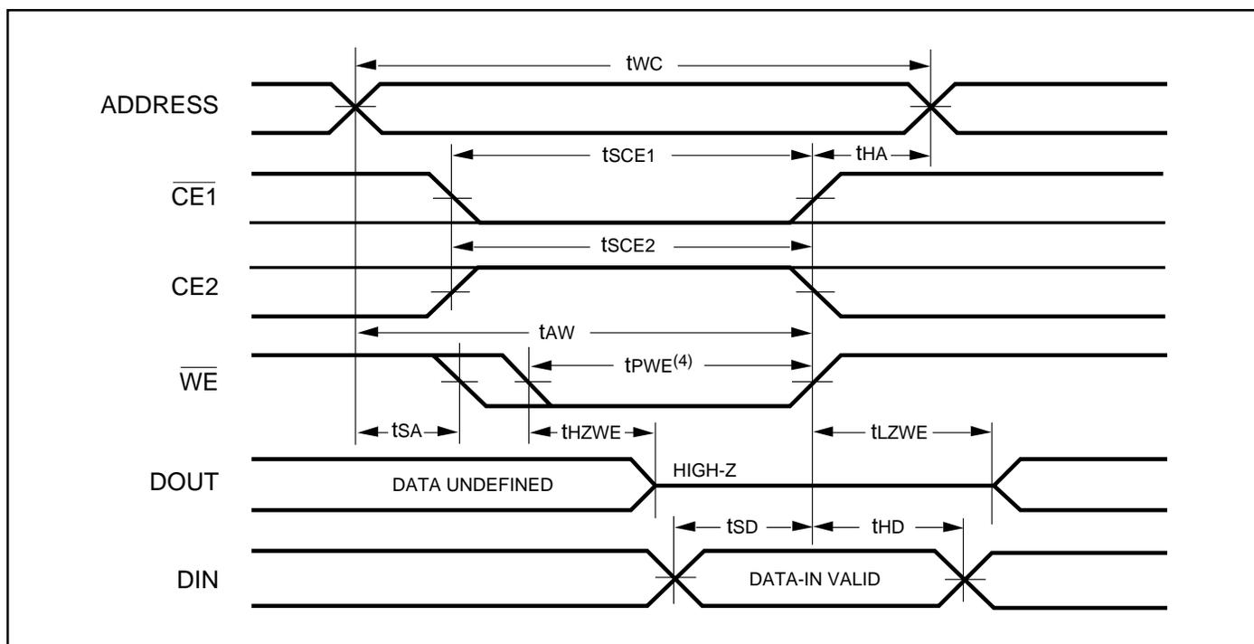
WRITE CYCLE NO. 2 ( $\overline{CE1}$ , CE2 Controlled)<sup>(1,2)</sup>
