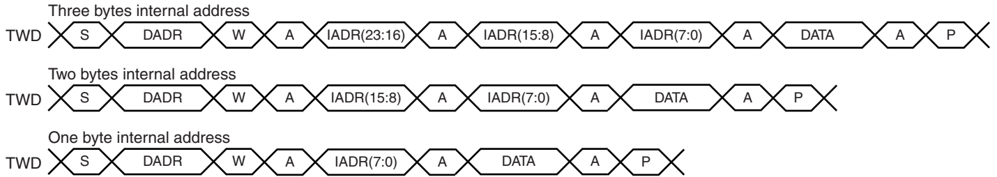
Figure 31-11. Master Write with One, Two or Three Bytes Internal Address and One Data Byte
