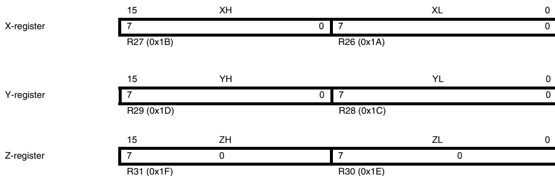
Figure 4-3. The X-, Y-, and Z-registers
