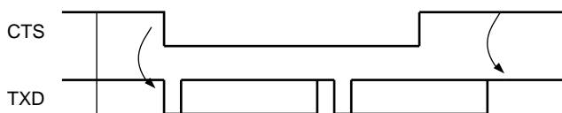
Figure 25-28. Transmitter Behavior when Operating with Hardware Handshaking
