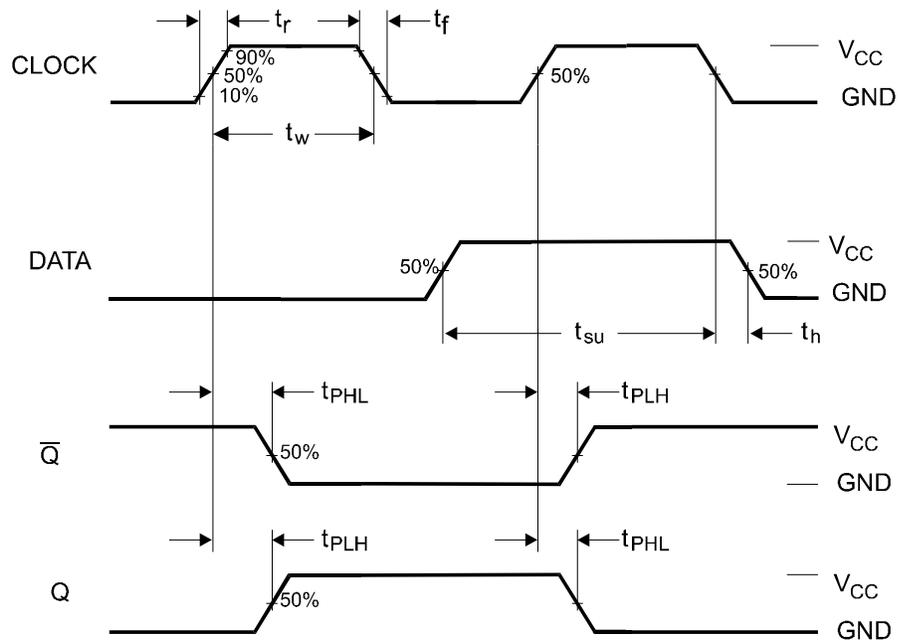
Figure 1. Switching Waveforms
