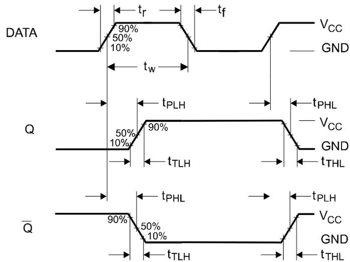
Figure 2. Switching Waveforms
