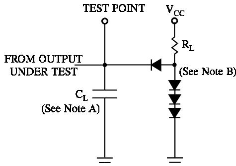
NOTES A.  $C_L$  includes probe and jig capacitance.
