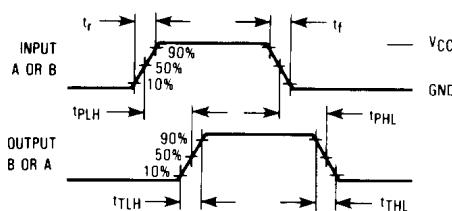
Figure 1. Switching Waveforms
