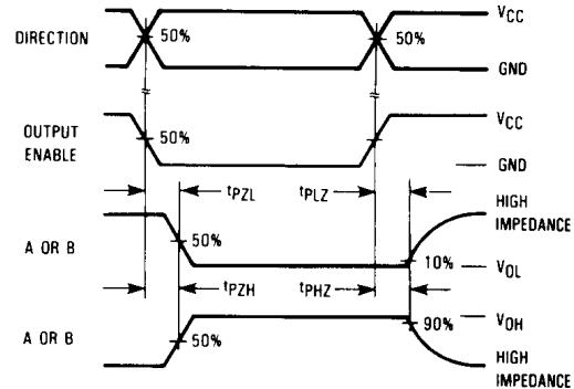
Figure 2. Switching Waveforms
