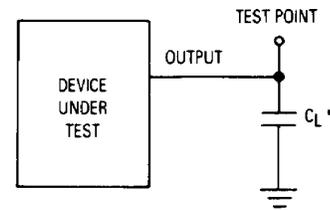
\*Includes all probe and jig capacitance.
