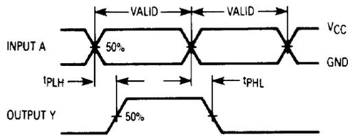
Figure 1. Switching Waveforms
