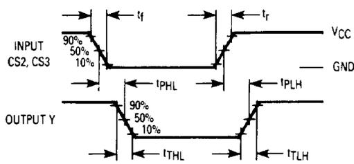
Figure 3. Switching Waveforms
