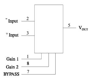
$\begin{aligned} & Pin \ 4 = GND \\ Pin \ 6 = Supply \ Voltage \ V^{+} \end{aligned}$
