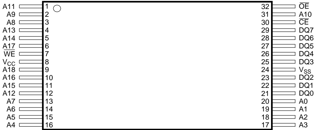
29F040 Standard Pinout
