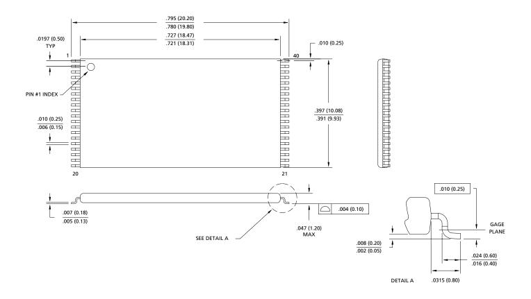
**NOTE:** 1. All dimensions in inches (millimeters) MAX or typical where noted.
