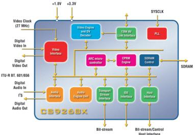
The new CS9268X is a family of single-chip, real time MPEG-2 audio and video encoders with an integrated DV decoder, DV to MPEG transcoder, system multiplexor, programmable VBI extraction, and a rich set of interfaces, such as IDE and IEEE 1394 link-layer A/V interface. The CS9268X family is designed for digital video recording systems, such as DVD recorders, personal video recorders, and advanced set-top boxes, as well as home media centers.
