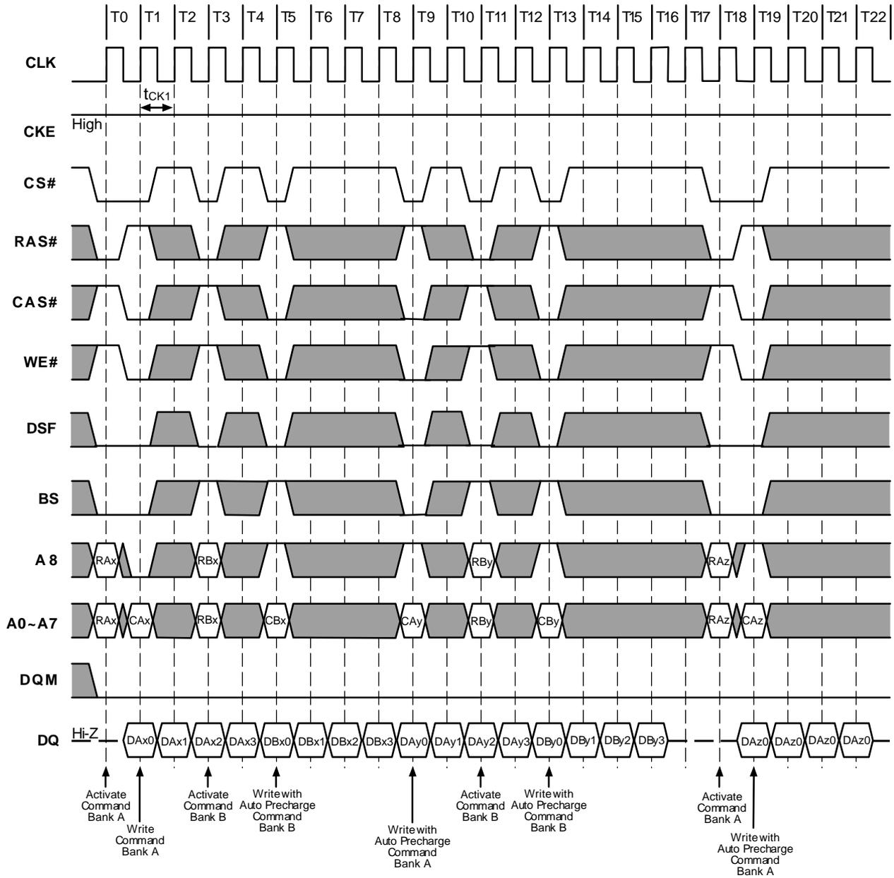
**Figure 17.2. Auto Precharge after Write Burst (Burst Length=4, CAS# Latency=2)**
