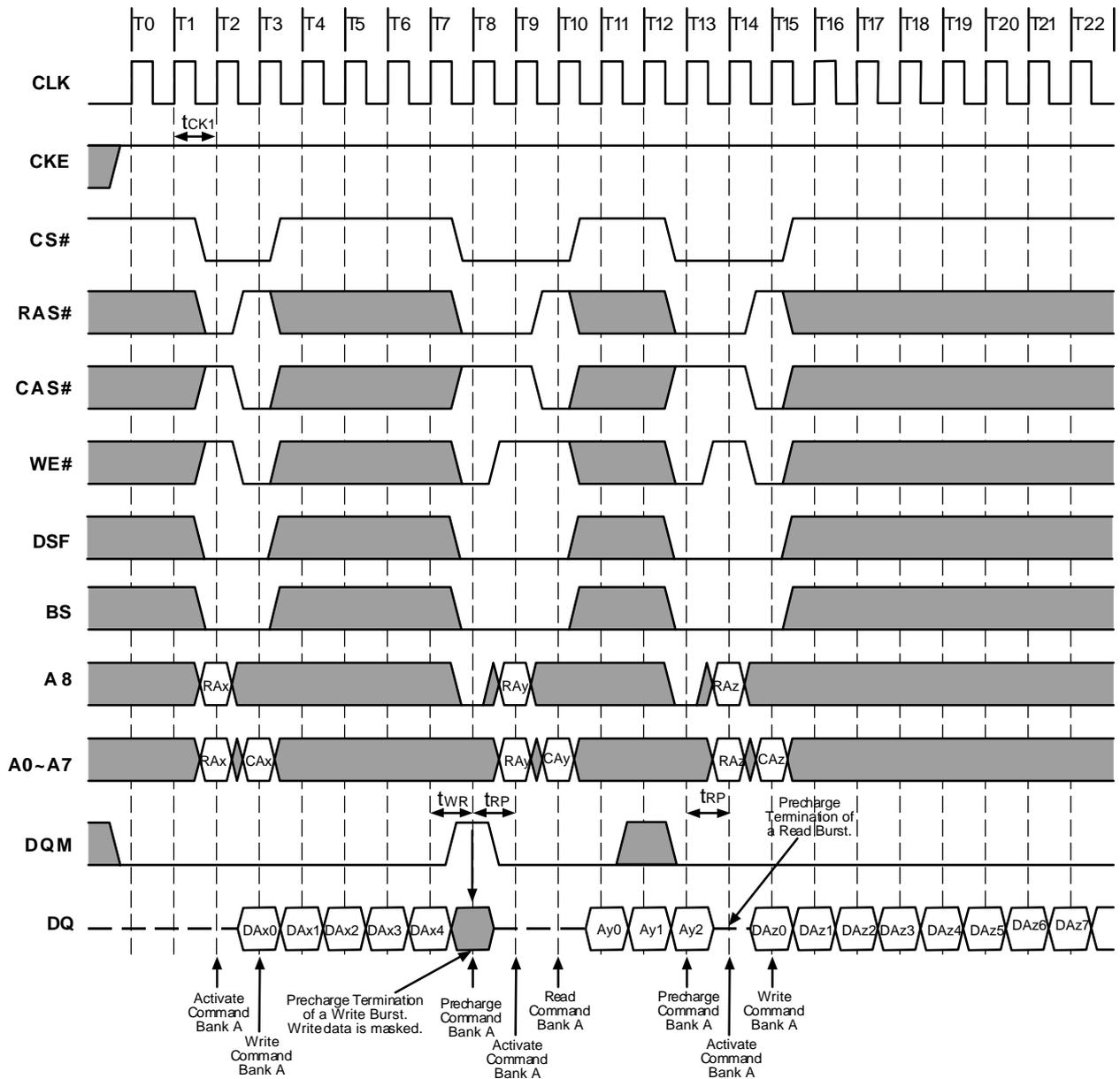
**Figure 26.2. Precharge Termination of a Burst**
