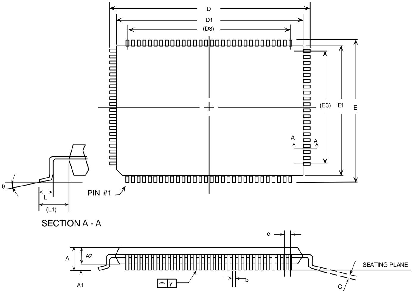
**TQFP1.4/QFP Packaging Dimensions**
