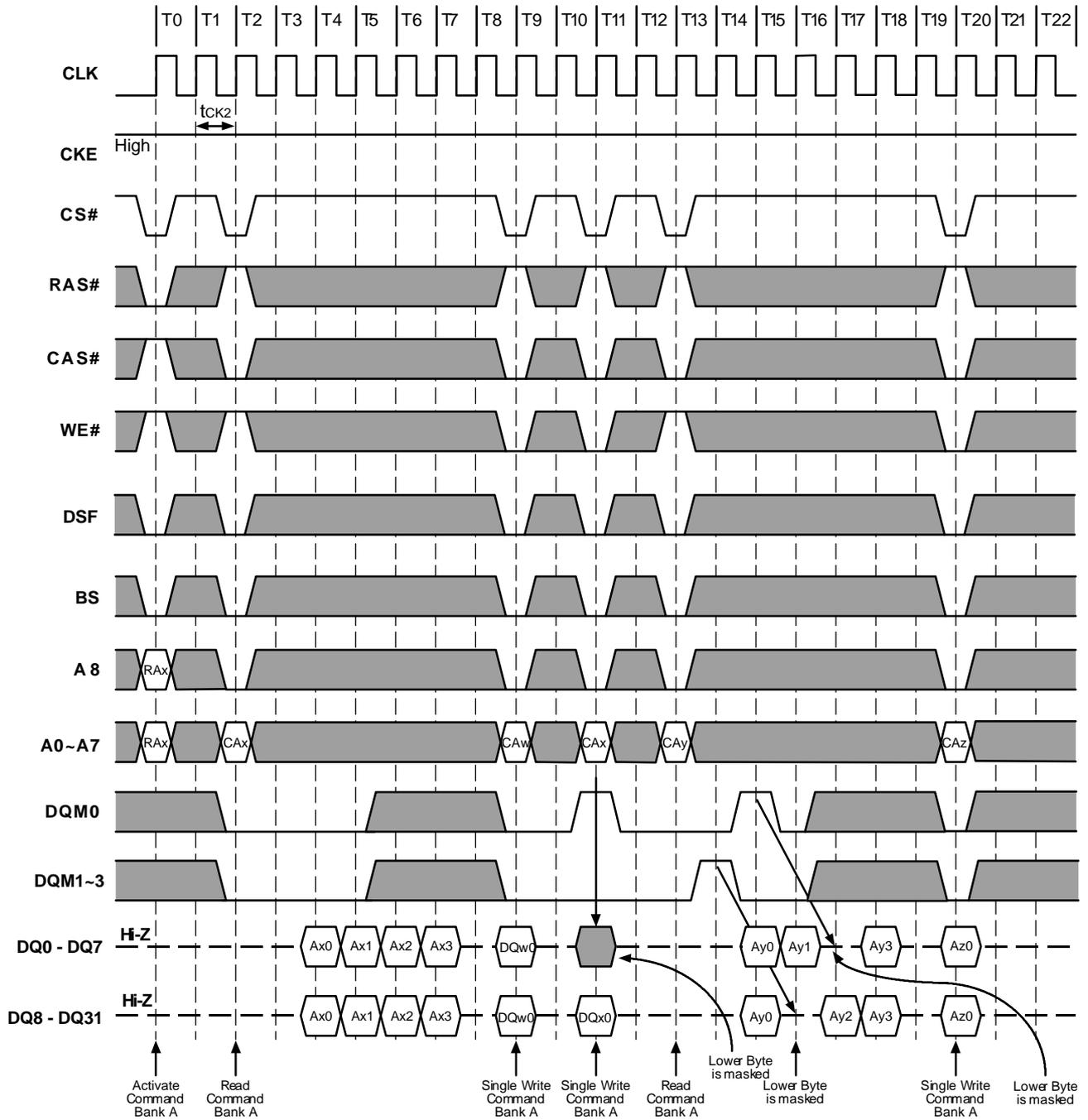
**Figure 22. Full Page Burst Read and Single Write Operation**
