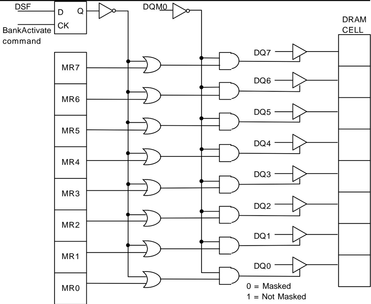
**Note:** Only the lower byte is shown. The operation is identical for other bytes.
