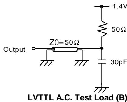
7. Transition times are measured between  $V_{IH}$  and  $V_{IL}$ . Transition (rise and fall) of input signals are in a fixed slope (1 ns).
