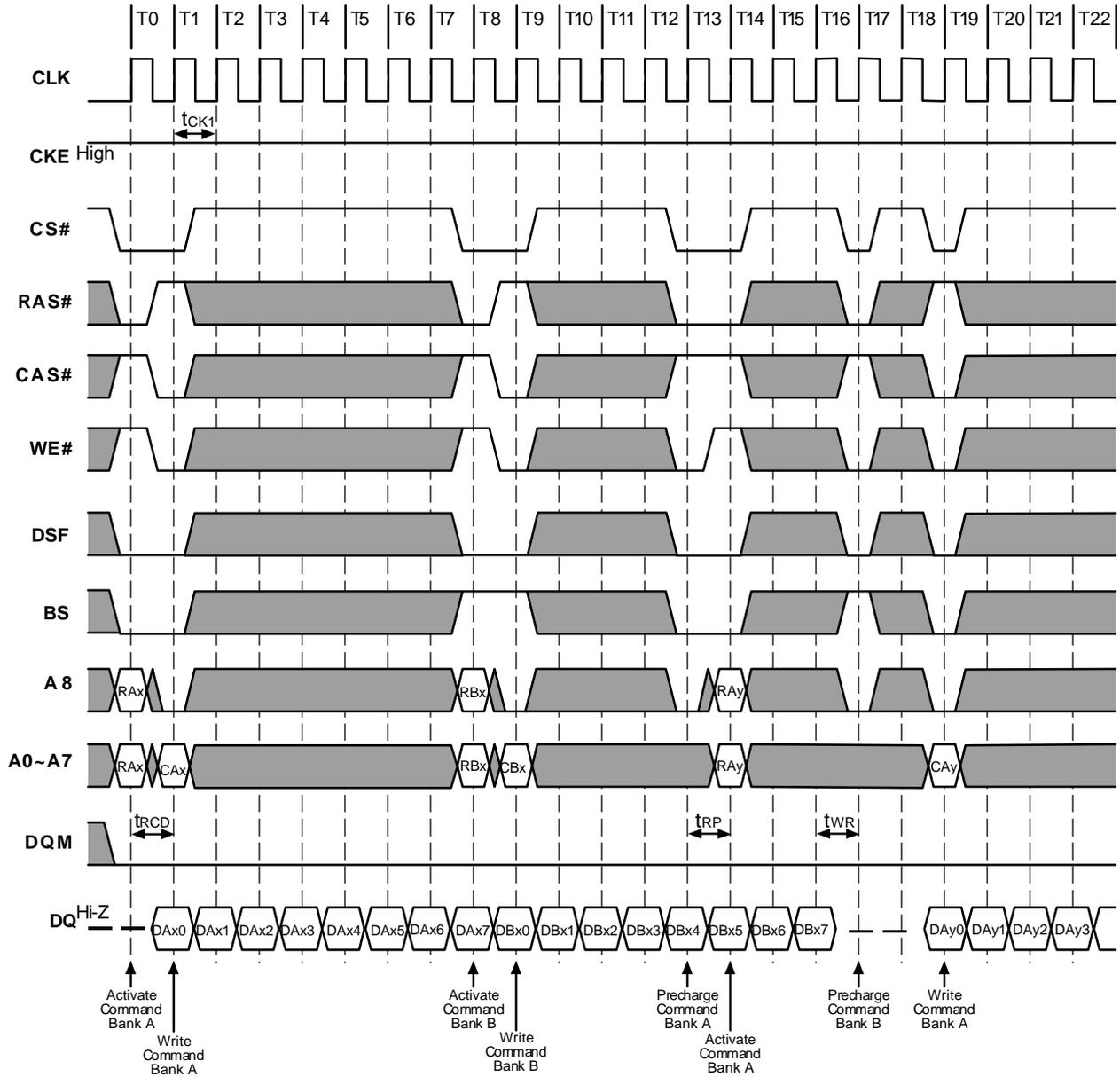
**Figure 12.2. Random Row Write (Interleaving Banks)**
