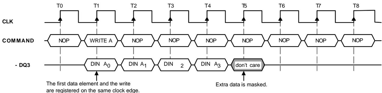
**Burst Write Operation (Burst Length = 4, CAS# Latency = 1, 2, 3)**
