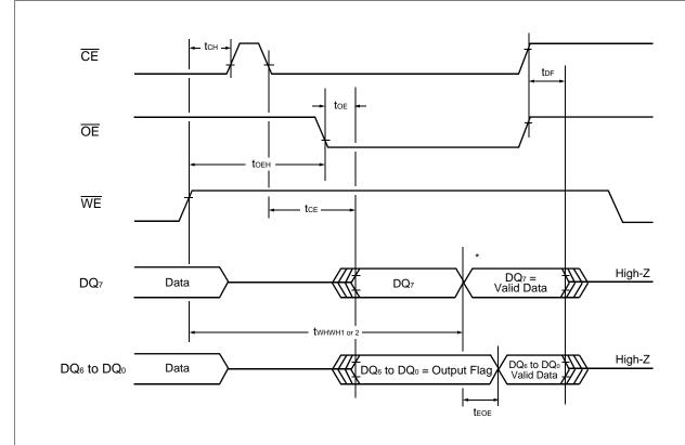
\* : DQ<sub>7</sub> = Valid Data (The device has completed the Embedded operation).
