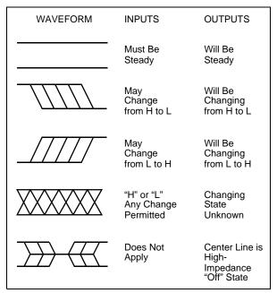
(1) AC Waveforms for Read Operations
