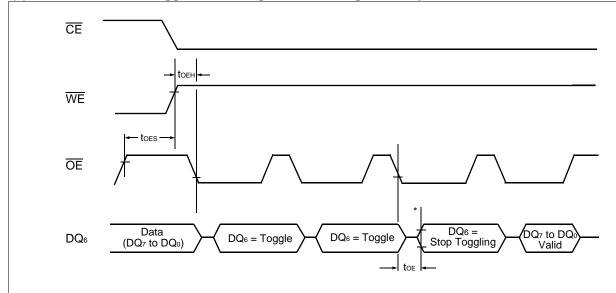
$^{\star}$  : DQ $_{\!6}$  stops toggling (The device has completed the Embedded operation).
