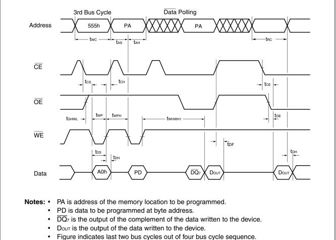
• These waveforms are for the ×16 mode. (The addresses differ from ×8 mode.)
