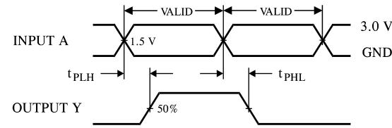
**Figure 2. Switching Waveform**
