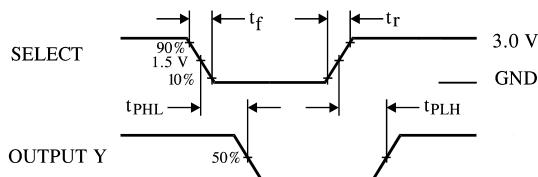
**Figure 1. Switching Waveform**
