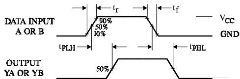
Figure 1. Switching Waveforms
