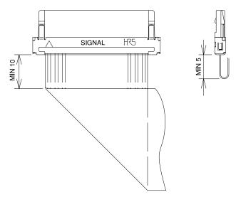
Note8:To assemble the FPC to the socket, use the recommended jigs and tools and be careful not to be injured by the edge of the metallic part of the connector. Observe the instructions given in the manual for wiring jigs and tools.
