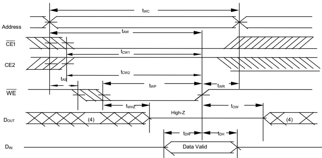
WRITE CYCLE 2 ( $\overline{CE1}$  and CE2 Controlled) (1,2,5)
