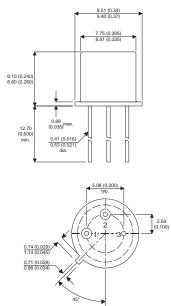
Bipolar NPN Device in a Hermetically sealed TO39
