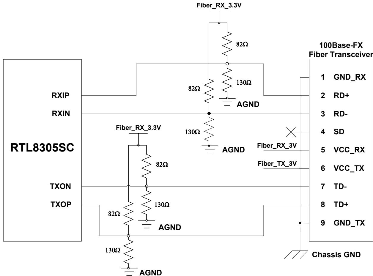
Figure 29. 100Base-FX with 3.3V Fiber Transceiver Application
