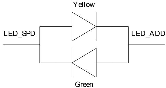
Figure 22. Two Pin Bi-color LED for SPD Floating or Pull-high
