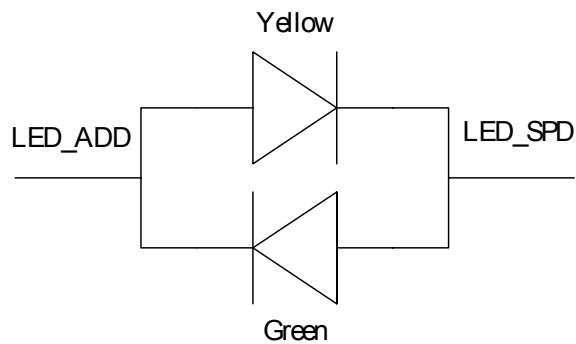
Figure 23. Two Pin Bi-color LED for SPD Pull-down
