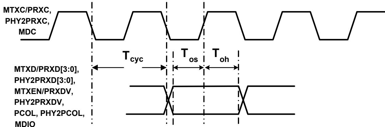
Figure 26. Transmission Data Timing of MII/SNI/SMI Interface
