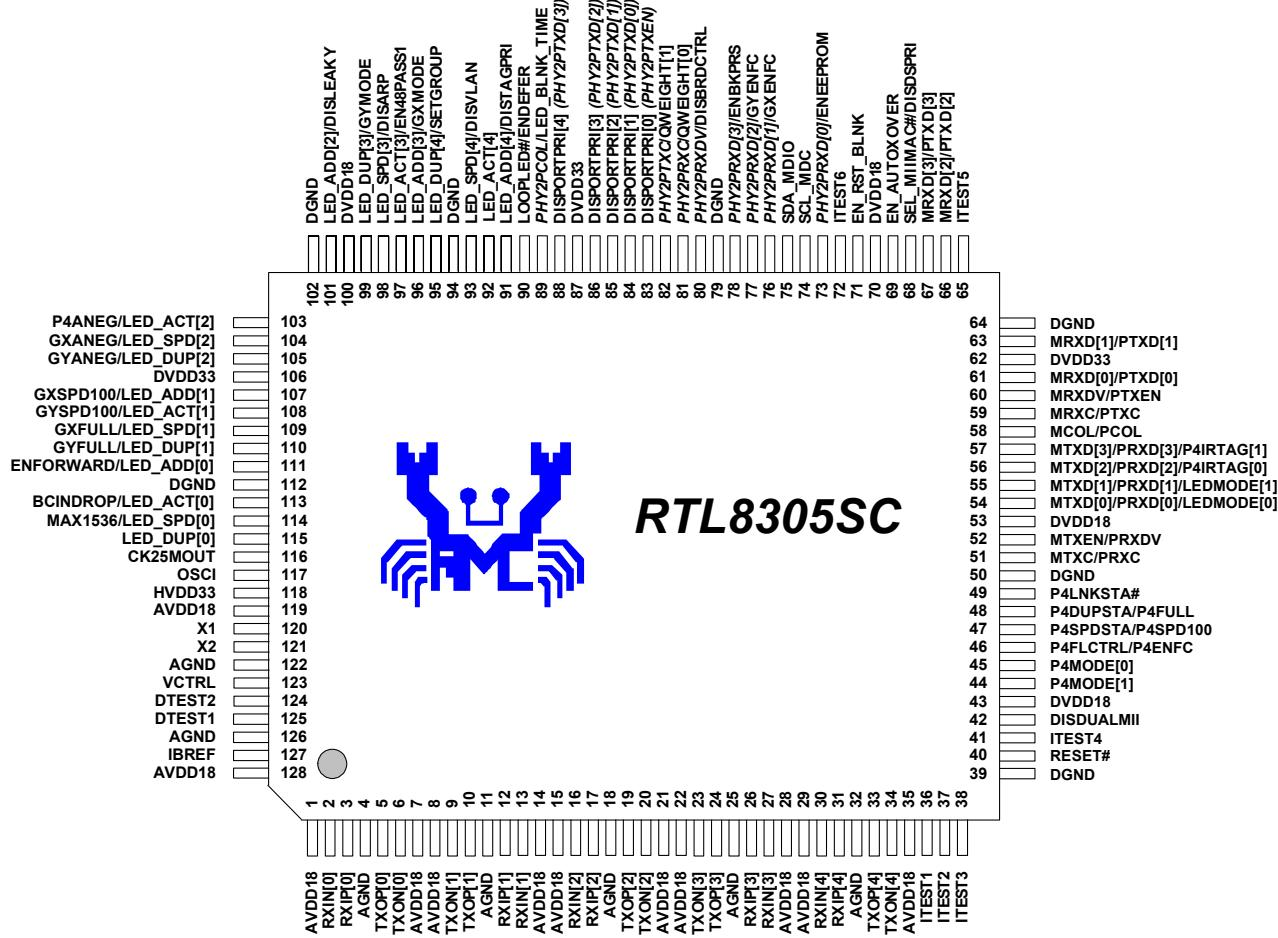
Figure 2. Pin Assignments
