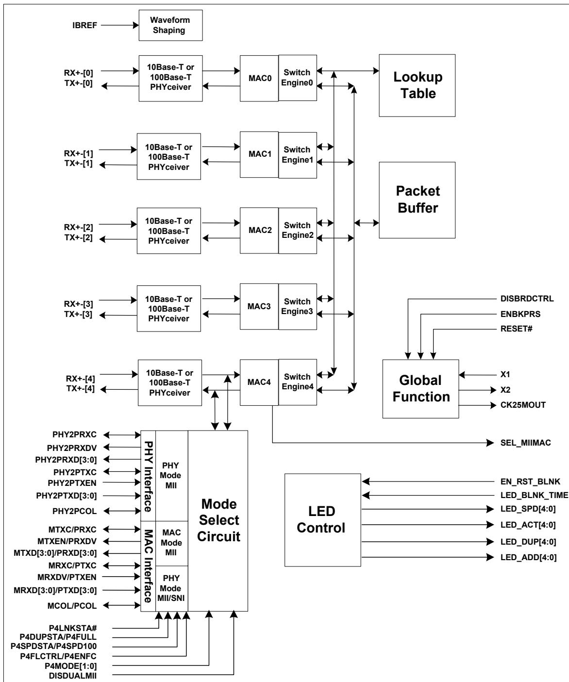
Figure 1. Block Diagram
