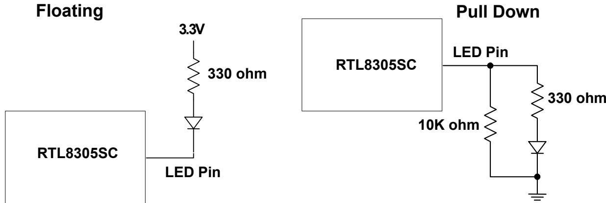
**Figure 21. Floating and Pull-Down of LED Pins**
