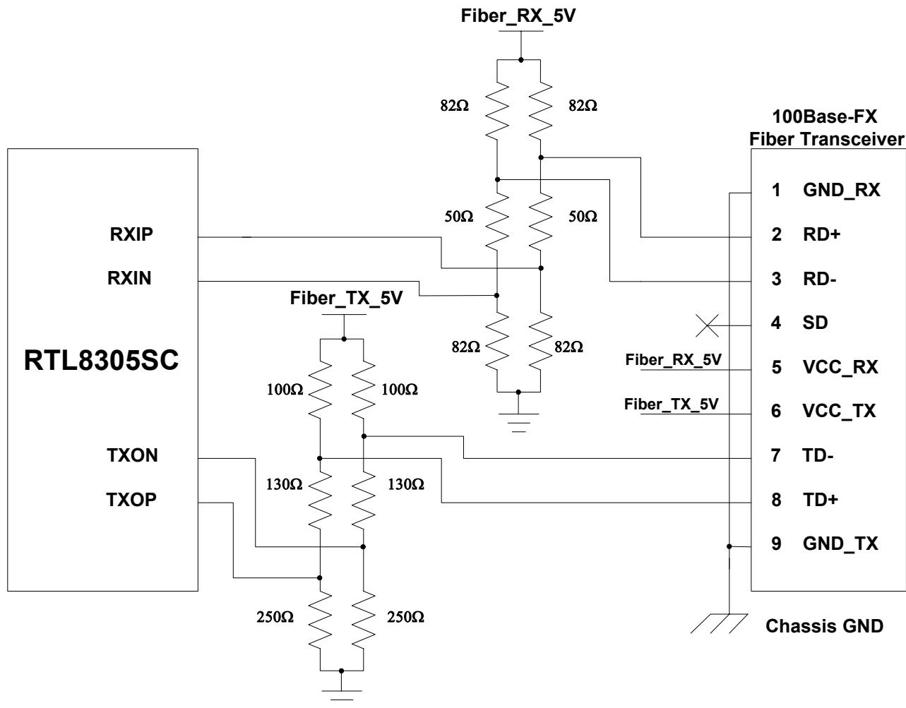
**Figure 30. 100Base-FX with 5V Fiber Transceiver Application**
