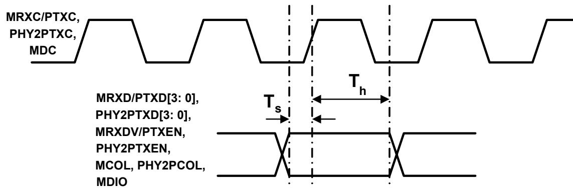
Figure 25. Reception Data Timing of MII/SNI/SMI Interface
