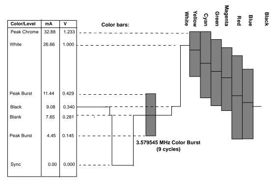
Figure 17: Composite NTSC Video Output Waveform (DACG = 0)
