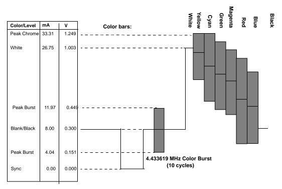
Figure 18: Composite PAL Video Output Waveform (DACG = 1)
