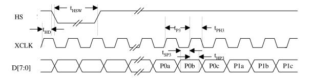
Figure 6: Multiplexed Pixel Data Transfer Mode (IDF = 6)
