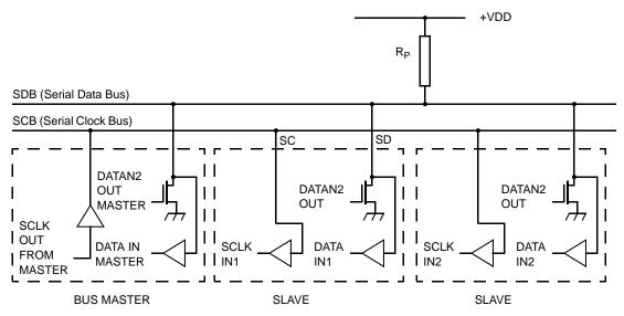
Figure 19: Connection of Devices to the Bus
