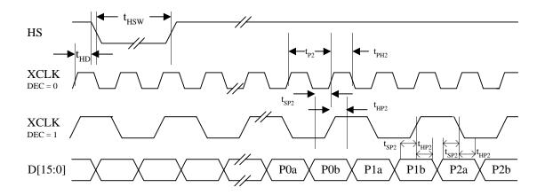
Figure 5: Multiplexed Pixel Data Transfer Mode
