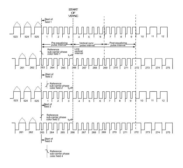
Figure 11: Interlaced NTSC Video Timing
