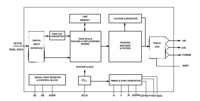
Figure 1: Functional Block Diagram
