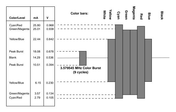
Figure 15: NTSC C (Chrominance) Video Output Waveform (DACG = 0)
