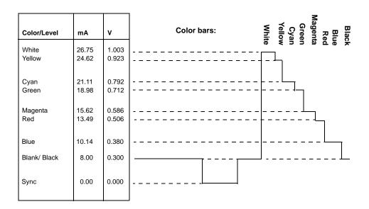
Figure 14: PAL Y (Luminance) Video Output Waveform (DACG = 1)
