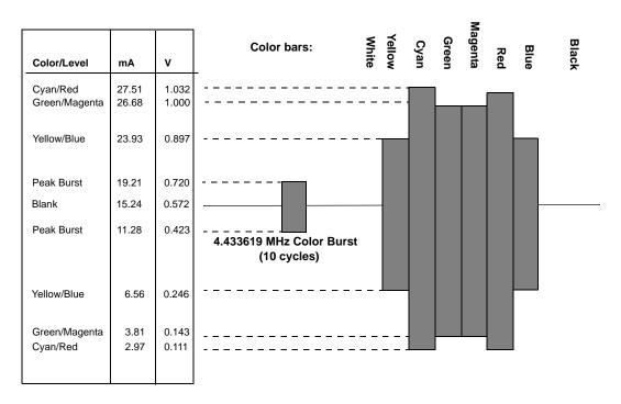
Figure 16: PAL C (Chrominance) Video Output Waveform (DACG = 1)
