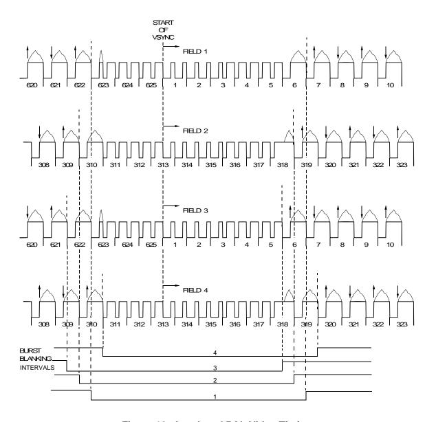
Figure 12: Interlaced PAL Video Timing
