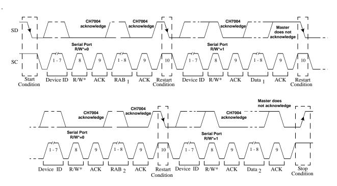
Figure 24: Alternating Read Cycle
