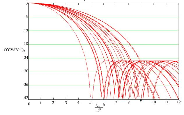
Figure 7: Composite Luminance Frequency Response (YCV = 0)
