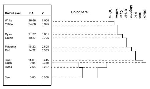
Figure 13: NTSC Y (Luminance) Output Waveform (DACG = 0)
