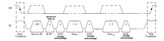
Figure 20: Serial Port Transfer Protocol
