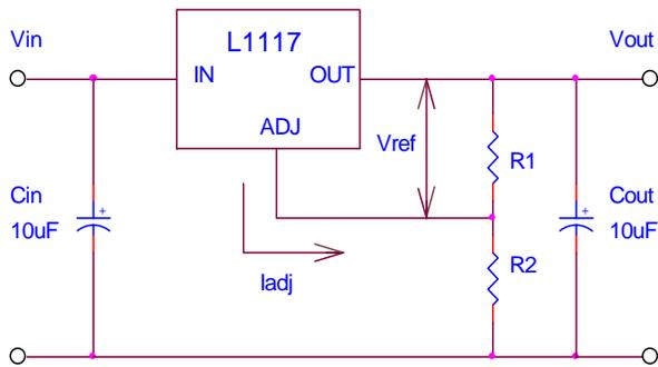
$$V_o = V_{ref} (1 + R_2/R_1) + I_{adj} \times R_2$$
