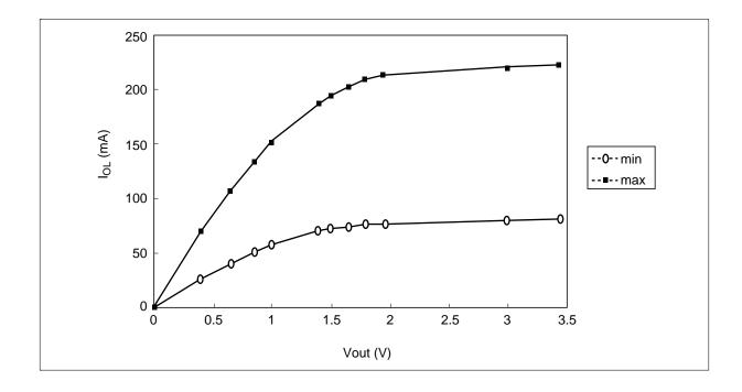
Output High Current ( $I_{OH}$ ) (Ta = 0 to +70°C,  $V_{CC}$ ,  $V_{CC}$ Q = 3.0 V to 3.45 V,  $V_{SS}$ ,  $V_{SS}$ Q = 0 V)
