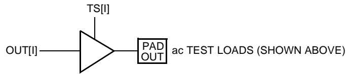
Figure 74. ac Test Loads
