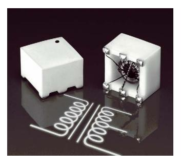
These wideband RF transformers were developed specifically for use with Analog Devices digital to analog high-speed converters and provide excellent performance at a very economical price. They come with a tapped secondary and are packaged in a low profile, flat top ceramic case that makes them ideal for pick and place operations. They feature 400 V isolation and a 500 mA maximum current rating. Operating temperature range is -40°C to +85°C.
