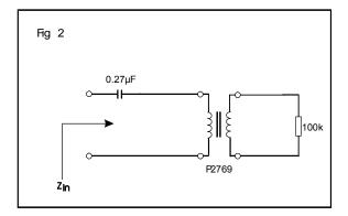
In practice, the  $100k\Omega$  load can be increased without limit. The DC blocking capacitor should be a minimum of  $0.22\mu F$  to avoid resonance within the voiceband to obtain a flat frequency response and input impedance to specification.
