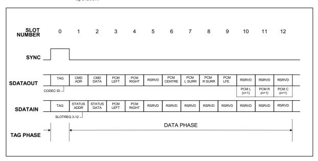
Figure 8 AC'97 Standard Bi-directional Audio Frame
