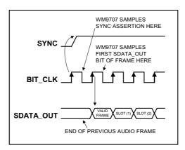
Figure 10 Start of an Audio Output Frame
