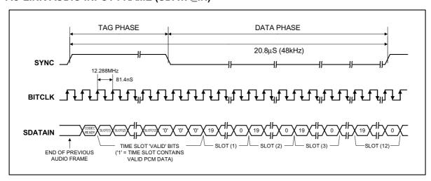
Figure 11 AC-link Audio Input Frame
