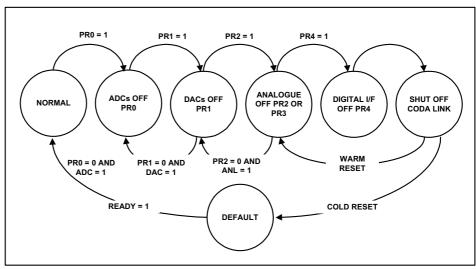
Figure 13 An Example of the WM9708 Powerdown/Powerup Flow
