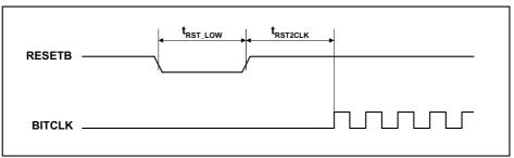
Figure 2 Cold Reset Timing
