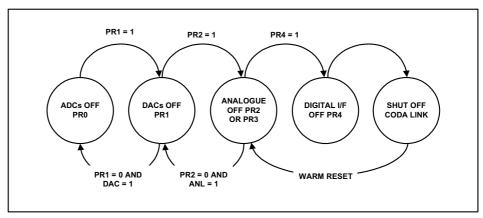
Figure 14 The WM9708 Powerdown/Flow with Analogue Still Alive
