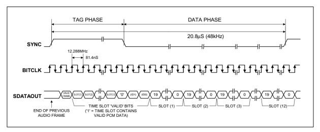
Figure 9 AC-link Audio Output Frame
