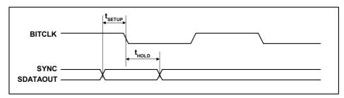
Figure 5 Data Setup and Hold (50pF External Load)
