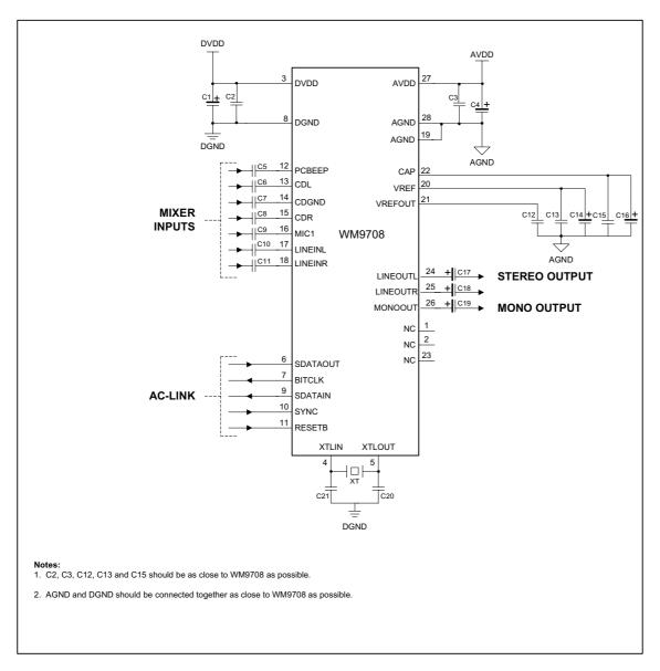
Figure 15 External Components Diagram
