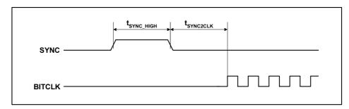
Figure 3 Warm Reset Timing
