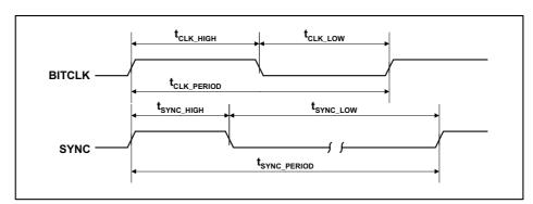
Figure 4 Clock Specifications (50pF External Load)
