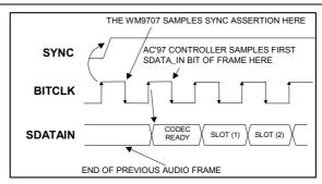
Figure 12 Start of an Audio Input Frame
