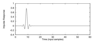
Figure 13 Impulse Response (Normal Roll-off, no De-emphasis)
