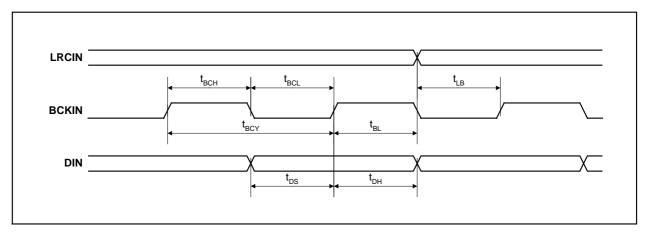
Figure 1 Audio Data Input Timing
