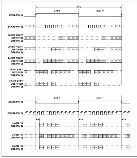
Figure 4 Audio Data Input Format
