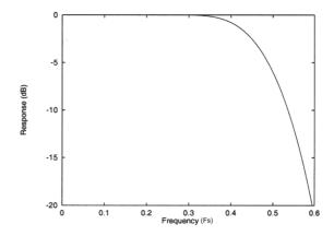
Figure 10 Digital Filter Response (Slow Roll-off Mode)
