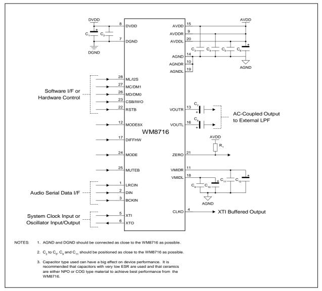
Figure 15 External Components Diagram
