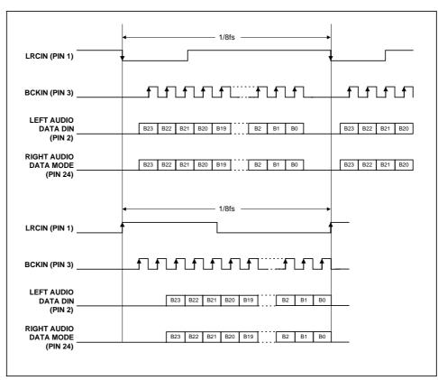
Figure 5 Audio Data Input Format (8 x fs Operation)
