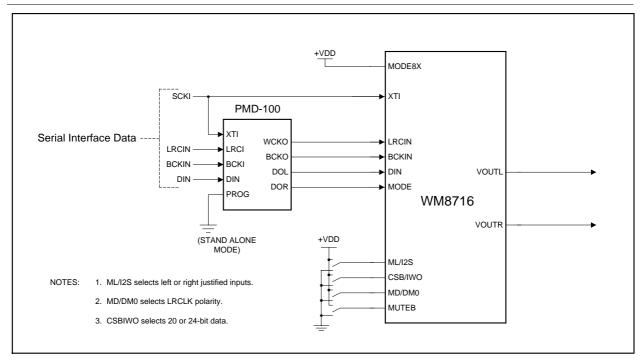
Figure 17 Example of WM8716 in MODE8X Operation
