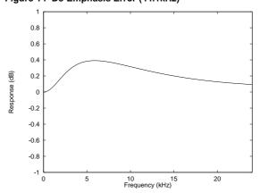
Figure 15 De-Emphasis Frequency Response (48kHz)
