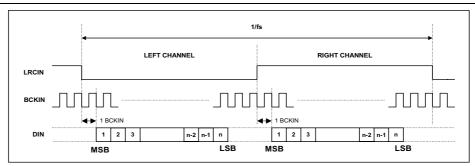
Figure 3 I<sup>2</sup>S Mode Timing Diagram
