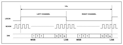
Figure 4 Right Justified Mode Timing Diagram
