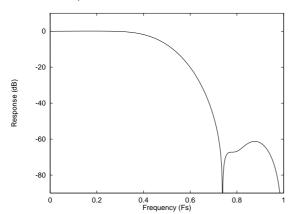
Figure 9 DAC Digital Filter Frequency Response -192kHz
