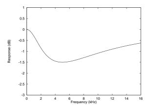
Figure 11 De-Emphasis Frequency Response (32kHz)
