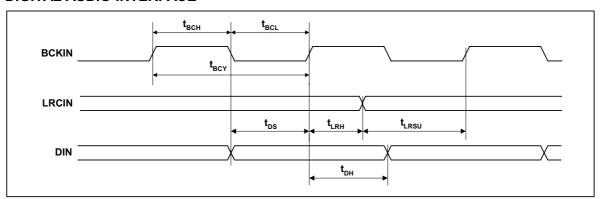
Figure 2 Digital Audio Data Timing
