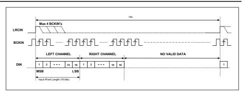
Figure 5 DSP 'Late' Mode Timing
