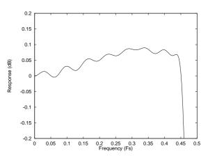
Figure 8 DAC Digital Filter Ripple
