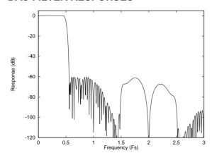
Figure 7 DAC Digital Filter Frequency Response -44.1, 48 and 96kHz
