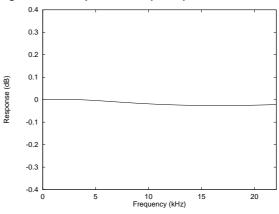
Figure 13 De-Emphasis Frequency Response (44.1kHz)
