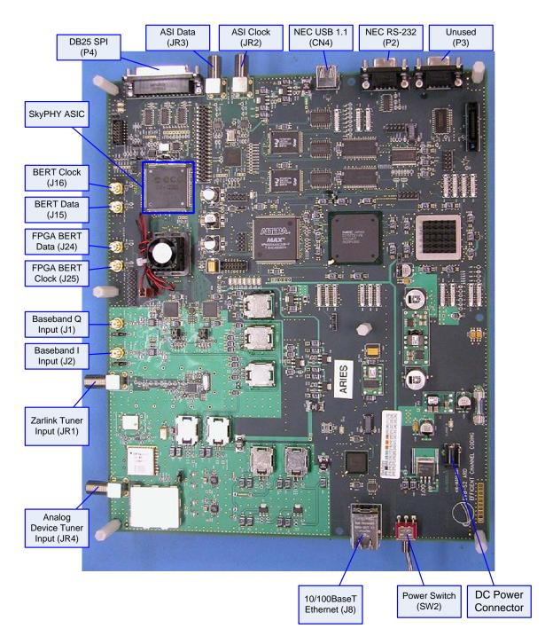
The evaluation board is designed for use in a lab environment. Care should be taken to ensure antistatic precautions are taken when handling the board. Electrostatic shock, excessive heat and moisture may cause damage to the board and attached components.
