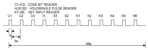
Basic transmitting waveform is 12-bits serial data in configuration as shown above.
