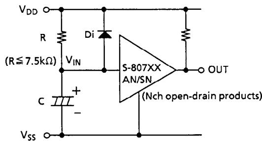
Note 1:  $R$  should be  $7.5k\Omega$  or less for purpose of protection against oscillation.
