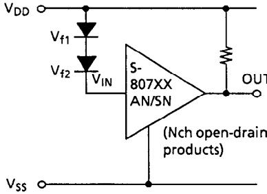
$$\text{Detection voltage} = V_{f1} + V_{f2} + -V_{DET}$$
