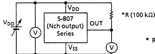
\* R is unnecessary for CMOS output products.
