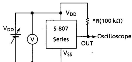
\* R is unnecessary for CMOS output products.
