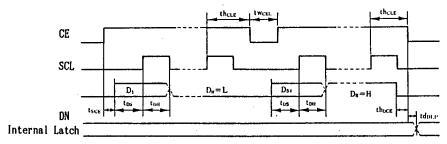
The data is latched at  $D_{\text{R}}\text{-H}$  and falling edge of the CE signal condition.
