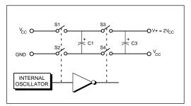
Figure 1. Charge Pump Voltage Doubler
