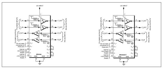
Figure 4. Typical Circuits using the SP233ACP and SP233ACT
