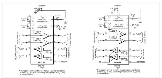
Figure 5. Typical Circuits using the SP310A and SP312A
