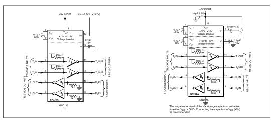
Figure 3. Typical Circuits using the SP231A and 232A.
