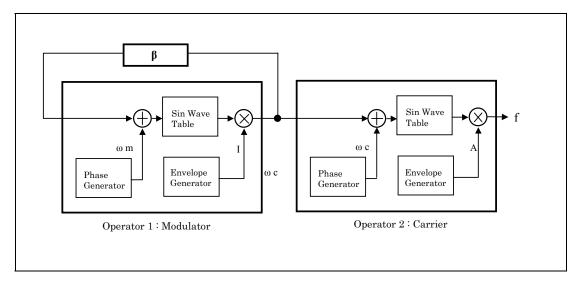
The "Operator" refers to the section where a sine wave is generated and the combination of the operators is called "algorithm". The operator in the front stage is called "modulator" and that in the rear stage "carrier". Each operator is capable of setting the frequency and the envelope waveform. The configuration in the above diagram can be expressed in the formula as follows.
