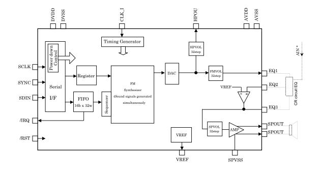
Concerning AIN signal inputted into equalizer circuit
