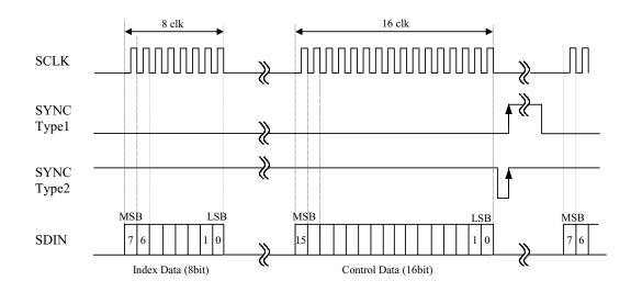
The YMU757B is controlled through the three serial interfaces SCLK, SYNC and SDIN.
