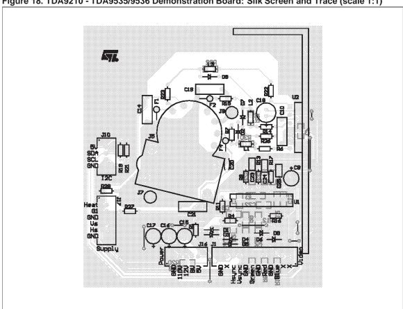
Figure 18. TDA9210 - TDA9535/9536 Demonstration Board: Silk Screen and Trace (scale 1:1)
