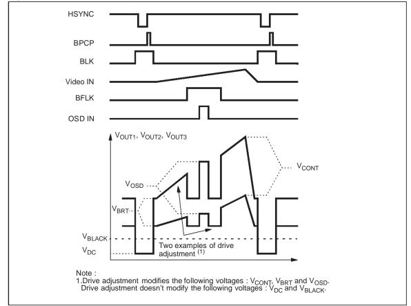
Figure 4. Waveforms (Drive adjustment)
