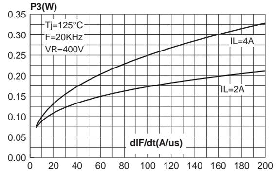
Fig. 7: Switching ON losses versus dIF/dt.
