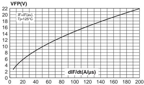
**Fig. 16:** Forward recovery time versus  $dI_F/dt$  (90% confidence).
