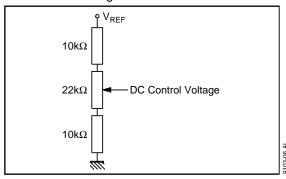
The input currents of the DC control inputs are typically very low (about a few  $\mu$ A). Depending on the internal structure of the inputs, the input currents can be positive or negative (sink or source).
