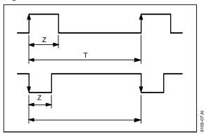
Using internal integration, both signals are recognized on condition that  $Z/T \le 25\%$ . Synchronisation occurs on the leading edge of the rectified signal. The minimum value of Z is  $0.7\mu s$ .
