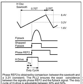
The phase comparator of PLL2 is similar to the one of PLL1, it is followed by a charge pump with a
