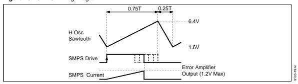
Figure 20: H Scanning Amplitude Regulation Example
