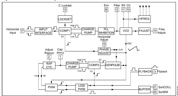
The PLL2 ensures the coincidence between the leading edge of the shaped flyback signal and a phase reference signal obtained by comparison of the sawtooth of the VCO and a constant DC voltage (3.2V) (see Figure 15).
