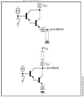
The output Darlington is in off-state when the power scanning transistor is also in off-state.
