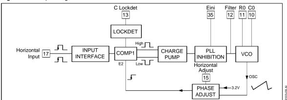
The dynamic behaviour of the PLL is fixed by an external filter which integrates the current of the charge pump. A "CRC" filter is generally used.
