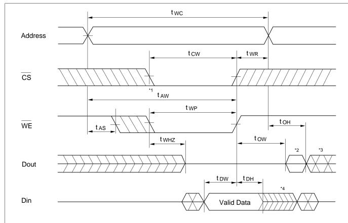
Notes: 1. If the  $\overline{\text{CS}}$  low transition occurs simultaneously with the  $\overline{\text{WE}}$  low transition or after the  $\overline{\text{WE}}$  transition, the output remain in a high impedance state.
