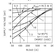
Supply Voltage vs R<sub>LOAD</sub> for Various V<sub>OUT</sub> (PDIP Package)
