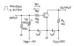
$I_{C}=10I_{B1}=-10I_{B2}=5A$  (For PNP, the polarity is reversed.)
