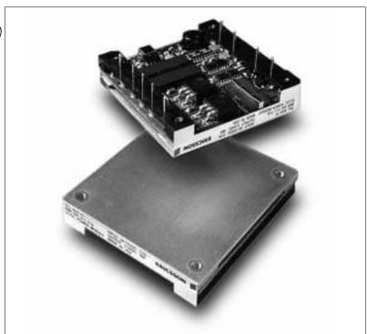
The PKJ 4000B series represents another one of Ericsson's "industry first" achievements in the continued development of our "Third Generation" of high-density, high-efficiency power modules. This module packs 48.2 W/in³ at 92% efficiencies (3.3V @ 40A) in an industry standard half-brick package. These breakthrough features come from using the most advanced patented topology utilizing integrated magnetics and synchronous rectification on a low-resistivity multilayer PCB.
