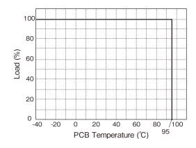
When using with different measurement conditions from output derating by ambient temperature, use output derating by PCB temperature.
