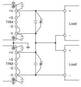
Fig.12-2 Series Operation due to ±Output
