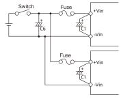
Fig.1-4 Input Filter when Plural Power Modules
