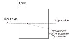
Fig.13-1 Measurement Point of Baseplate Temperature
