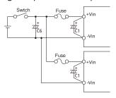
Fig.1-4 Input Filter when Plural Power Modules
