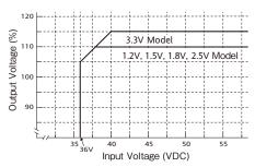
Fig.2-1 Limit of Input Voltage
