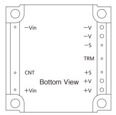
Input and Output Terminal Configurations(Bottom View)
