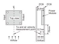
Fig.1-1 Output derating set-up condition
