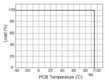
Fig.1-6 Output Derating by PCB Temperature
