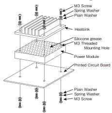
Fig.1-1 Mounting method for standard model
