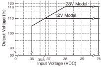
Fig.2-1 Limit of Input Voltage
