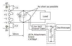
Fig.3-1 Measurement of Maximum Output Ripple & Noise
