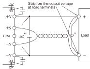
Fig.9-1 Remote Sensing is in Use
