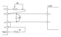
Fig.2-6 Example connection of external resistor
