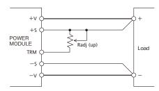
Fig.2-4 Connection for output voltage trim up
