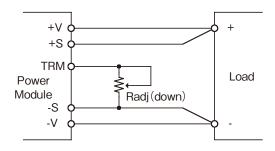
Fig.2-2 Connection for output voltage trim down
