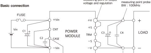
Note: This diagram is for Negative Logic "ON/OFF" Option.
