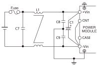
Fig.1-6 Recommended input filter as EMI countermeasure
