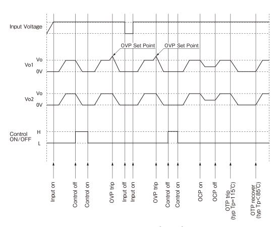
Note: This timing diagram is for Negative Logic "ON/OFF" Option.
