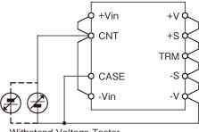
Withstand Voltage Tester
