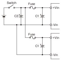
Fig.1-4 Input Filter when Plural Power Modules
