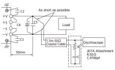
Fig.3-1 Measurement of Maximum Output Ripple & Noise
