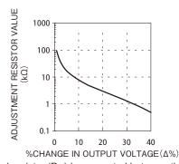
If the external resistor ( $R_{\mbox{\tiny adj}}$ ) is connected between the TRM pin and +S pin, the output voltage will increase. Diagram shown below is the output voltage trim up connection.
