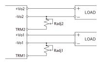
The equations and graphs for the required external resistor (Radi) value to obtain a percentage output voltage change of  $\Delta$  Vo% is as shown in the next page.
