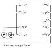
500VDC 1minute (10mA) Fig.19-2 Withstand Voltage Test for Output-Baseplate
