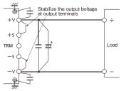
Fig.9-2 Remote Sensing is Not in Use
