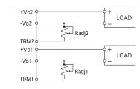
The equations and graphs for the required external resistor ( $R_{adj}$ ) value to obtain a percentage output voltage change of  $\Delta Vo\%$  is as shown in the next page.
