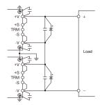
Fig.12-1 Series Operation due to High Output Voltage
