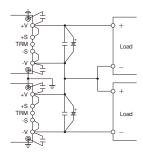
Fig.12-2 Series Operation due to ±Output
