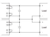
Fig.12-2 Series Operation due to ±Output
