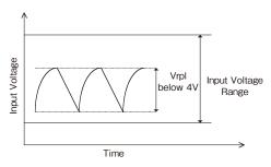
Fig.1-1 Input Ripple Voltage
