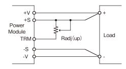
Fig.2-4 Connection for output voltage trim up
