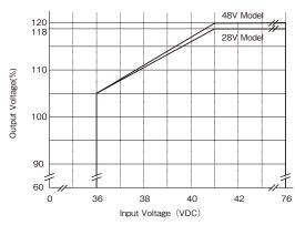
Fig.2-1 Limit of Input Voltage
