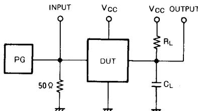
(1) The pulse generator (PG) has the following characteristics:
