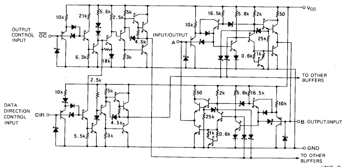
**OCTAL BUS TRANSCEIVERS WITH 3-STATE OUTPUTS(NONINVERTED)****ABSOLUTE MAXIMUM RATINGS** ( $T_a = -20 \sim +75^\circ\text{C}$ , unless otherwise noted)
