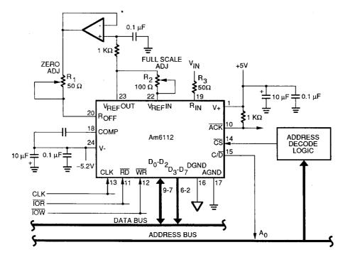
\*A low impedance Op Amp is recommended for optimum performance due to fast switching currents appearing at  $R_{OFF}\,.$
