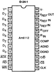
Note: Pin 1 is marked for orientation.
