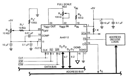
\*Remove  $R_2$  and make  $R_1 = 1 M\Omega$  for lowest noise, medium speed operation.
