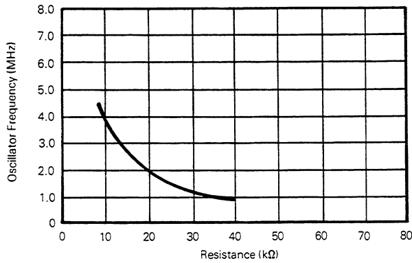
Figure 5-8. Typical Frequency Selection for Resistor Oscillator Option
