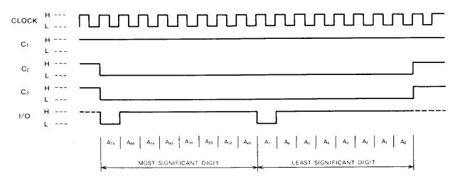
Note 2. The addresses from  $A_{00}$  to  $A_{77}$  are designated by two one-of-eight coded digits. The above figure shows designation of address  $A_{77}$
